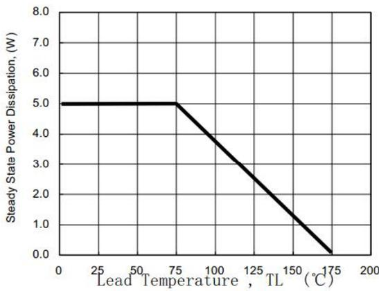
Fig. 3 - Steady State Power Derating Curve
