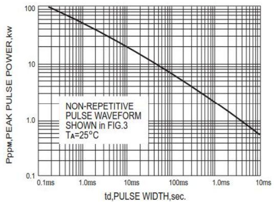
Fig. 4 - Peak Pulse Power Rating Curve
