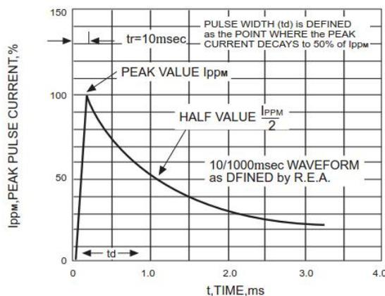
Fig. 5 - Pulse Waveform
