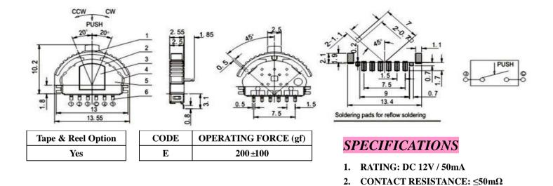
4. INSULATION RESISTANCE:  $\geq 100 M\Omega$
